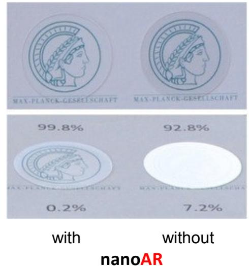
The newly-developed **nanoAR** process makes affordable production on a large scale possible. Applications include high power laser systems, optical sensing systems, touchscreen displays and devices, spectroscopy systems, potential stealth applications, light extraction and light harvesting devices.
